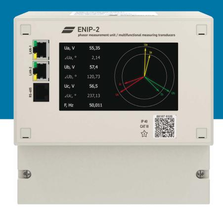
ENIP-2 phasor measurement unit (PMU) integrates into Wide Area Measurement Systems (WAMS) used for detection and prevention of instabilities in power grid networks as well as for power grid monitoring.
