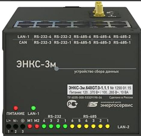
2 x LAN, USB, 6 x RS-485, 4 x RS-232, CAN, GPRS, GPS
